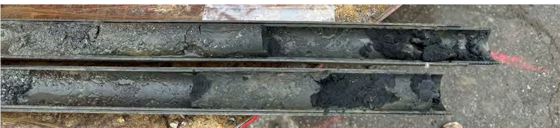
SPT Split Spoon Sample S-6 at Test Boring B-3 (15 to 17 ft BGS)
