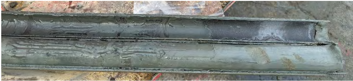
SPT Split Spoon Sample S-9 at Test Boring B-3 (30 to 32 ft BGS)
