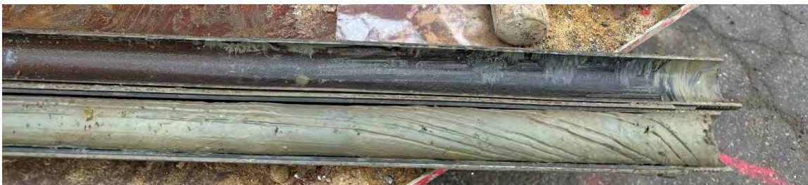
SPT Split Spoon Sample S-5 at Test Boring B-3 (10 to 12 ft BGS)
