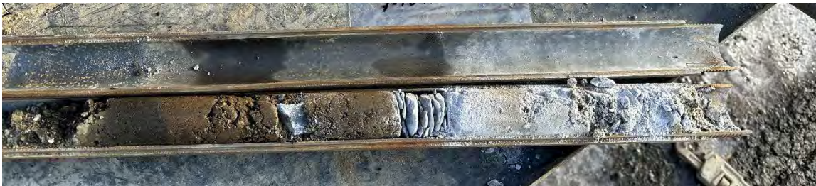
SPT Split Spoon Sample S-1 at Test Boring B-4 (1 to 3 ft BGS)
